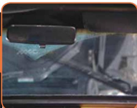
If the wiper blades are not wiping the glass evenly, or are smearing the windshield, you will need to replace the blades.
