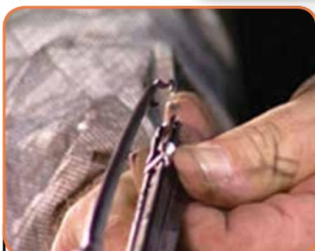
Remove the blade assembly. Depending on the vehicle, you may need to remove the wiper arm from its mounting...
