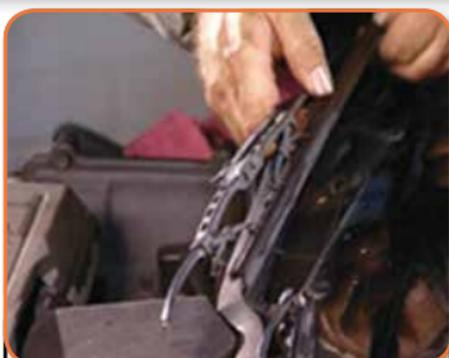
...or you may be able to just undo a spring clip and remove the blade insert.
