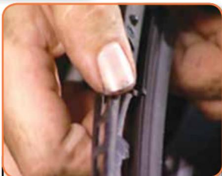
...and make sure the clips fit snugly and engage properly. Or refit a new blade assembly.
