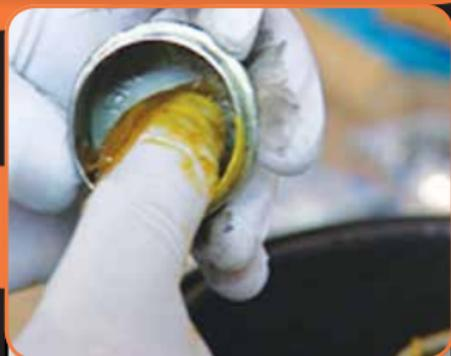
Also, pack some grease into the dust cap. Fill it about one-third, not all the way up.
