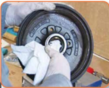
Clean out any grease in the hub, and dispose of the grease in an environmentally friendly manner.
