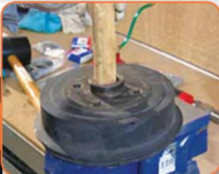
Using a long dowel or drift, and using a hammer gently drive on the front of the inner hub bearing from inside the hub unit.
