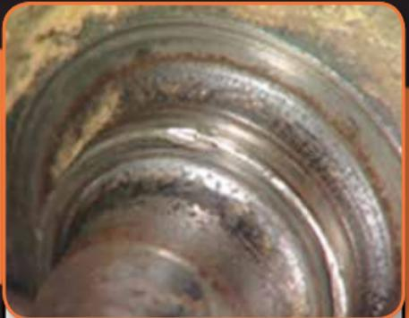
If the seal area is worn, grooved or damaged, it will affect the sealing function, the seal will need to be replaced.
