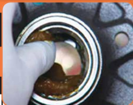
Put a small amount of grease in the cavity of the hub.
