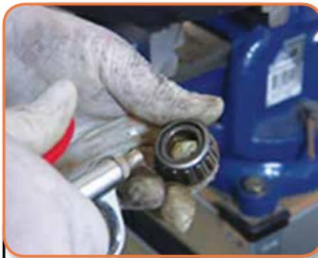
If you use an air blower as part of the cleaning process, be careful not to blow the old, dirty grease into the bearing or let the bearing spin.
