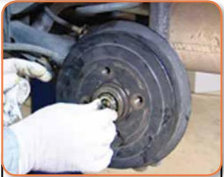
Put the outer bearing in place...
