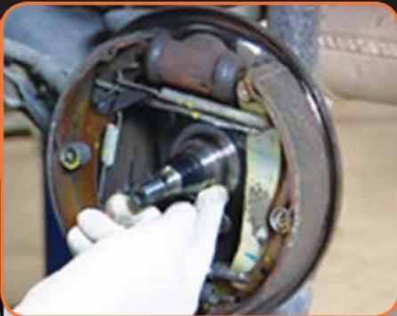
Inspect the sealing area for any signs of wear or damage.
