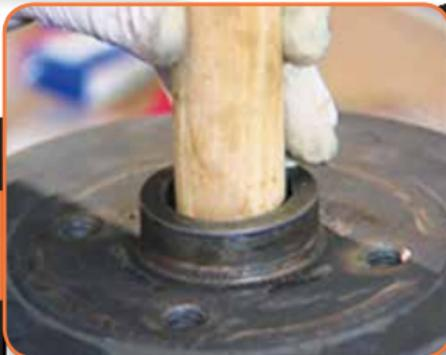
This will push the bearing out, and also remove the oil seal. It is good practice to renew the oil seal when you service the bearings.
