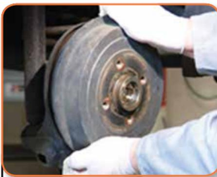
When removing the hub, be careful not to get any of the grease on the brake shoes if they are still in position.
