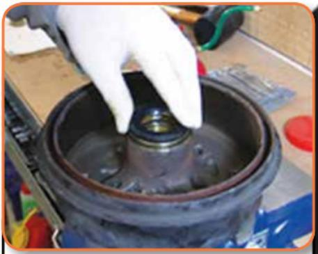
Install the new seal with its sealing lip facing towards the bearing, with a recommended seal-installing tool.
