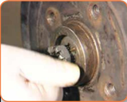
...add the washer and retaining nut, and screw it up by hand until it just touches the back of the outer bearing.
