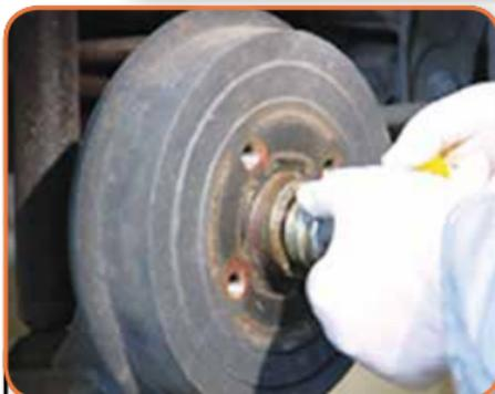
Pry off the dust cap, and remove the locking device. This is usually a cotter pin through the nut and spindle.
