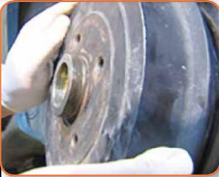
Slide the hub assembly onto the spindle and ensure it sits on the sealing area.
