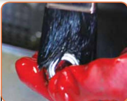
Clean the bearing with solvent, and air dry on a paper towel or blow it dry with compressed air.
