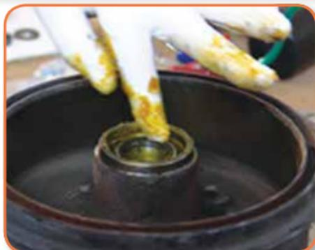
Re-install the bearing. Leave a ring of grease below the bearing race to help keep the fresh grease inside the bearing area after it heats up.
