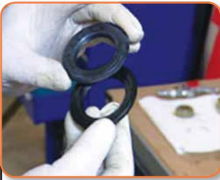
Before installing the new seal, ensure it is the right size to go over the spindle, by checking its diameter with the old oil seal that was removed from the hub.
