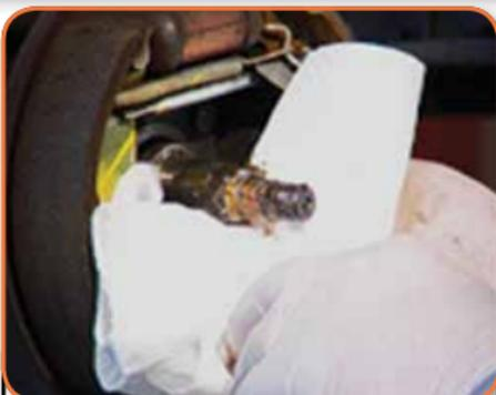
Use a paper towel to wipe all of the old bearing grease from the spindle, and the hub dust cap.
