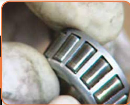
If you see any pitting or obvious damage, replace the bearing and the bearing race. These must be replaced as a set.
