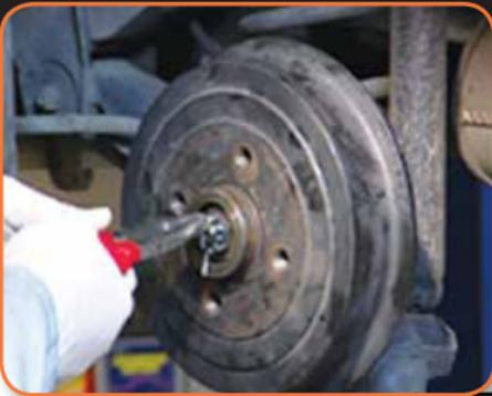
Re-install the brake assembly and check that the job is secure and within manufacturer's specifications prior to replacing the road wheel.
