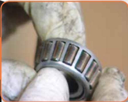
Inspect the bearing and its housing, which is called the "bearing race," for damage.
