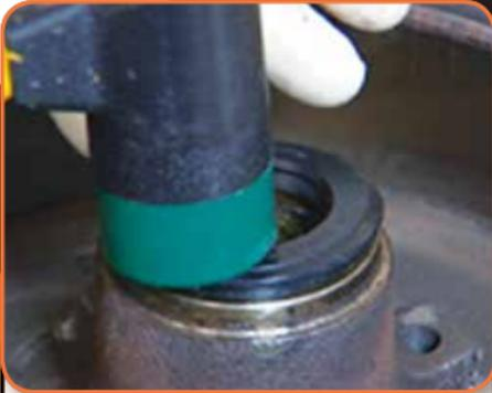
Carefully tap on the installer tool ensuring that the seal goes in straight.
