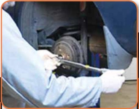
Now tighten, or pre-load the bearing, in accordance with the specifications in the vehicle's manual.
