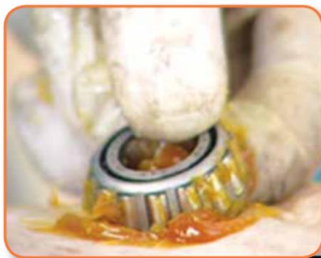
Work the grease into the large open end of the bearing until it oozes out the opposite side, then spread a fresh layer of grease all around the bearing...
