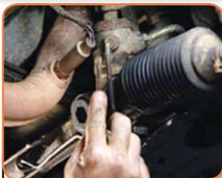
Inspect both the steel lines and the flexible hoses for any signs of deterioration.
