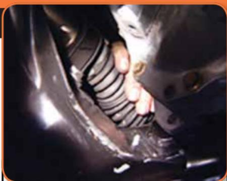
Inspect the rubber boots for any signs of being torn or damaged. If torn or dislodged from its seat, dirt or abrasives may have entered the unit, accelerating wear.
