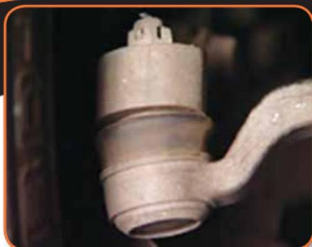
If the ball and socket is worn, there will be a noticeable movement in the tie-rod assembly.
