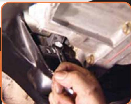
...and check the tightness of these mounting bolts.
