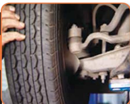
As the wheel assembly is moved by this rocking action, note any excessive movement in the front tie-rod end.
