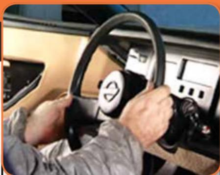
With the vehicle raised, have an assistant turn the steering wheel from side to side.
