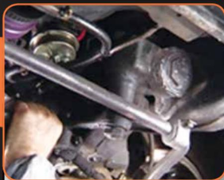
A steering system of the parallelogram type is normally fitted with a steering box assembly. You should check for excessive movement in the steering box itself.
