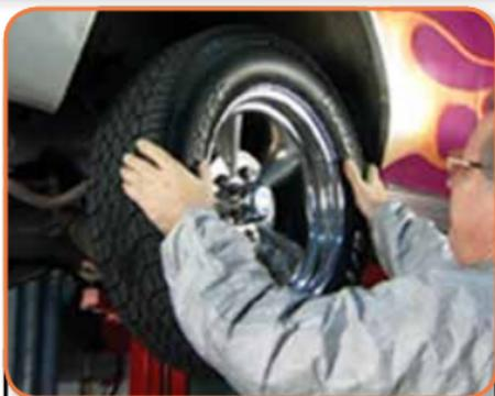
If the steering system is a parallelogram type, move the tyre/wheel assembly from side to side, and check the idler arm bush for excess movement.
