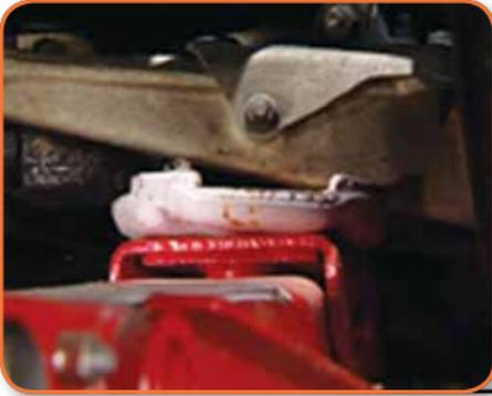
...and supported under the lower arms. This places the weight of the vehicle on the ball joints.
