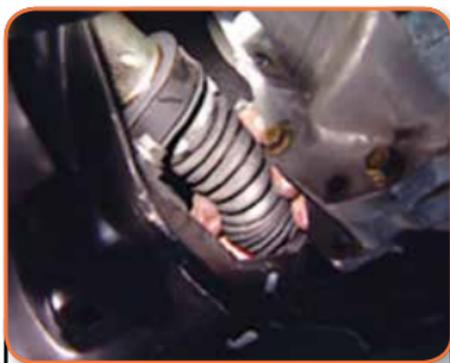
Squeeze the boots so that you make contact with the inner ball joint, and feel for any excess movement to check for wear in...
