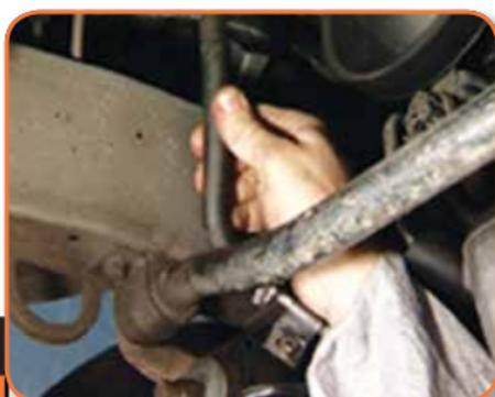
Chafing can necessitate the replacement of the lines, if rubbed through.
