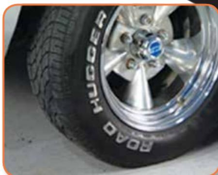
While watching the wheels, see how much you can move the steering wheel, before the wheels start to move.
