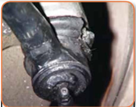
If torn or dislodged from its seat, dirt or abrasives may have entered the tie-rod end, accelerating wear in the unit.
