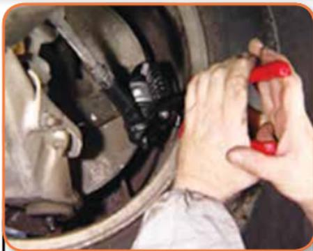
On a spring-loaded unit, one test is to compress the spring. Spring-loaded sockets should have a firm spring pressure when compressed all the way.
