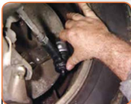
There are two basic types of tie-rod ends, spring-loaded and pre-loaded.
