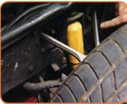
In the case of a torsion bar, or a long arm/short arm type suspension, where the spring is acting on the lower arm, you can test ball joints by having the vehicle raised off the ground slightly...
