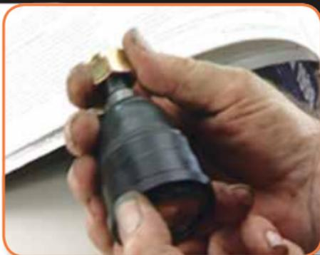
Some manufacturers add a wear indicator to their ball joints. The most common type of wear indicator has a shoulder that sticks out of the bottom of the joint by 1.27mm when new.
