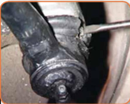
Inspect the rubber boot on the tie-rod end for any signs of being torn or damaged.
