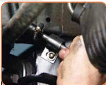
Check the steel lines for signs of chafing. If present, chafing is usually a sign of loose or missing locating clamps.
