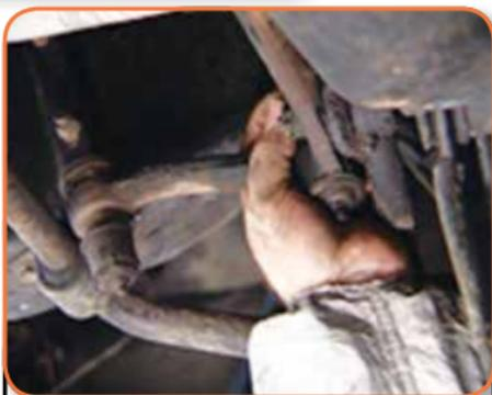
Alternatively, push and pull on the idler arm, at the same time checking movement in all of the pivoting points attached to the steering linkage.
