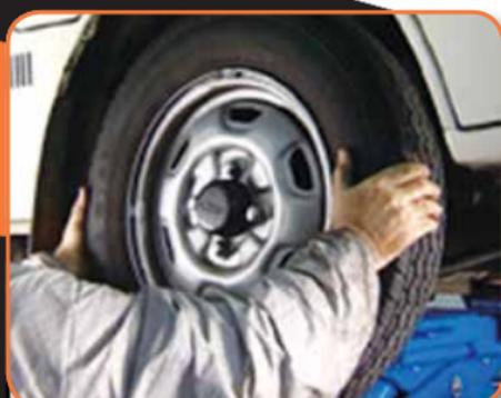
With the vehicle's weight off the steer wheels, move the tyre/wheel assembly from side to side.
