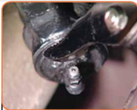
To check these types of joints use a large pair of channel lock pliers which are also known as multigrip type pliers, and place one jaw under the base of the ball joint...
