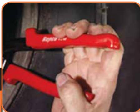
By squeezing the handles of the pliers, you should be able to see the movement inside the joint.
