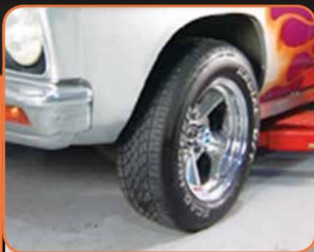
This can be done by having the vehicle on the ground, and feeling the "free play" in the steering wheel with the wheels in the straight ahead position.
