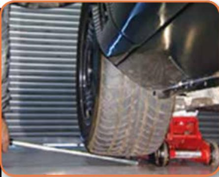
Now place a lever under the tyre and pull the tyre assembly up.
