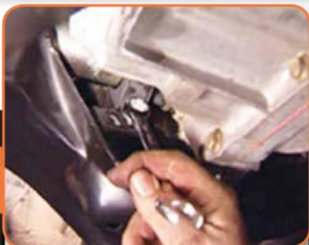
Check that the rack housing is securely mounted to the cross member...
