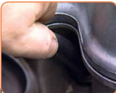
...by grasping the boot where it connects to the plug, twist it and pull it firmly straight out.
