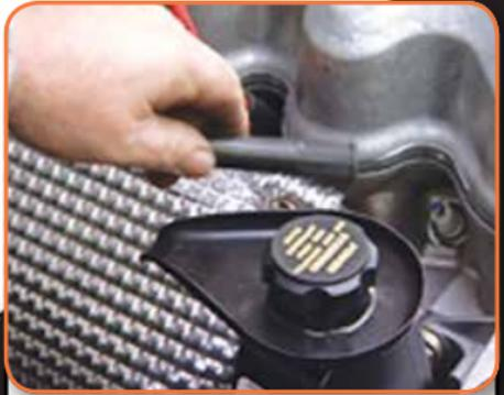
...and push it firmly into place over the exposed spark plug terminal.
