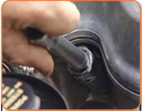
Turn the plug counter-clockwise to loosen it, and then turn the socket by hand until you can remove it.
