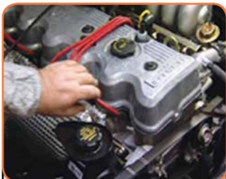
Before removing the spark plug, disconnect the spark plug high tension lead...
