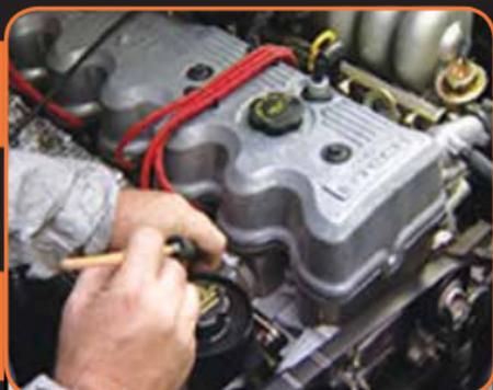
If possible, use a small paint brush to clean away any loose dirt or dust...
