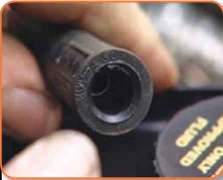
Apply some silicon lubricant to the inside of the boot at the end of the coil lead...
