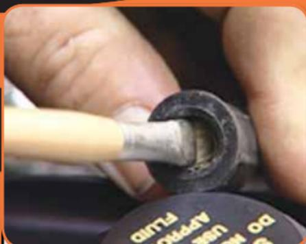
...gathered round the base of the plug, which may fall into the cylinder, when the plug has been removed.
