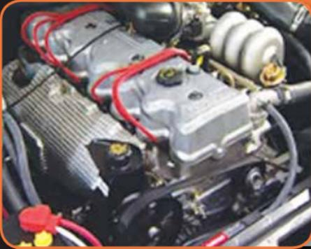
Start the engine to confirm that the plugs and leads are functioning correctly and that the engine is not misfiring.
