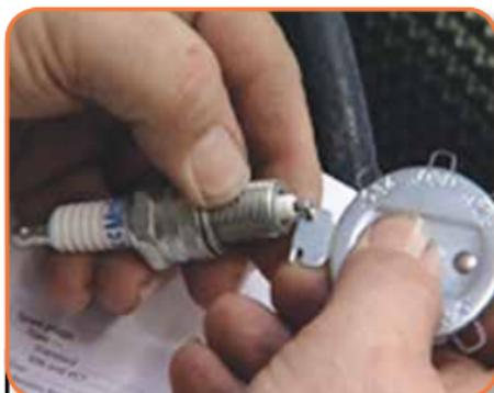
If the gap between the electrodes is too wide or too narrow, adjust it by bending the ground electrode with a gap-adjusting tool.
