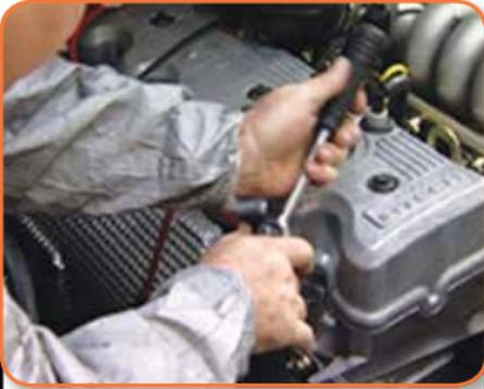
Spark plugs can sometimes be difficult to remove, so you may need to extend the wrench handle for additional leverage.
