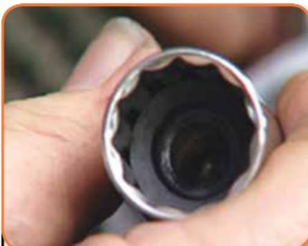
This usually has a rubber insert to protect the plug while it is being removed.
