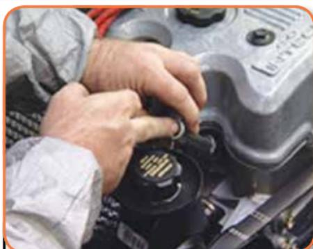
Replace the spark plug in its seat, carefully screwing it in by hand to avoid stripping the thread.
