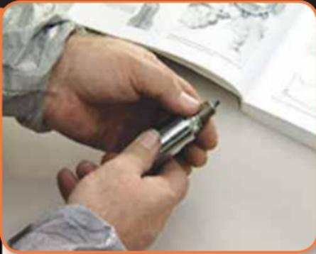
Remove the spark plug from the socket and clean it...
