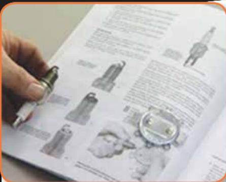
Check the condition of the plug. If the insulator is cracked, or the electrodes are burned or heavily corroded, or the thread is stripped, then the plug will need to be replaced.
