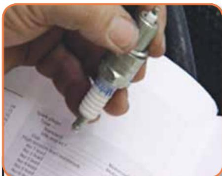
Check the plug specifications for the correct gap, and measure this with a wire gauge of the correct diameter.
