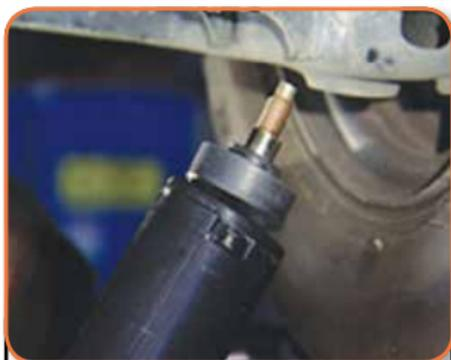
Fit the rubber mountings to both ends of the shock absorber...
