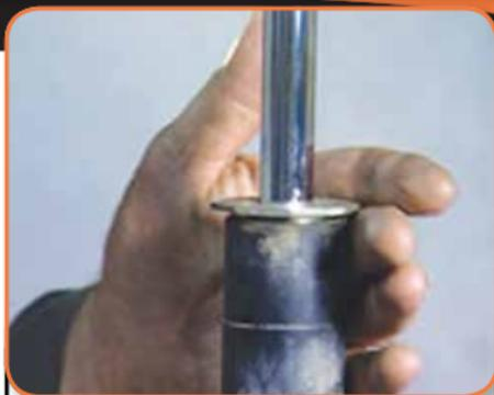
Loosen and remove the nut that locates the strut cartridge within the strut housing...
