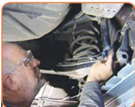
If the shock absorber is not integrated with the strut assembly, make sure the vehicle weight is supported...
