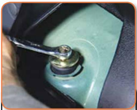
Tighten the fastener to the manufacturers recommended value.
