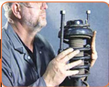
Remove the top mount and the upper spring cradle, and remove the spring.
