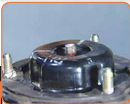
Loosen and remove the nut that secures the top mount to the shaft.
