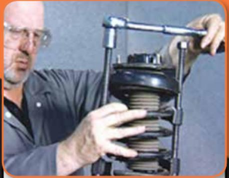
Loosen the spring compressor while guiding the spring into its correct position within the upper and lower cradle.
