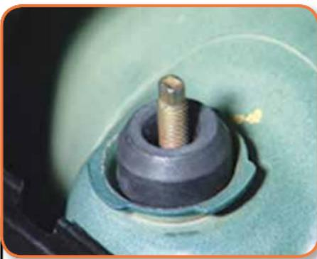
Fit the other half of the rubber mounts to the mounting boss and attach the fastener.
