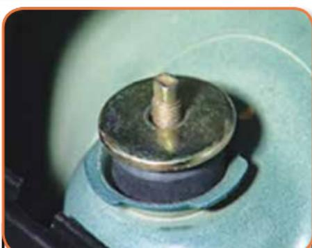
...and then loosen the fasteners at the top...
