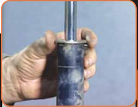
...and tighten the securing nut.
