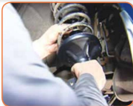
Refer to the manufacturers' manual and follow the instructions on how to refit the strut assembly. Repeat the procedure for the strut assembly on the other side.
