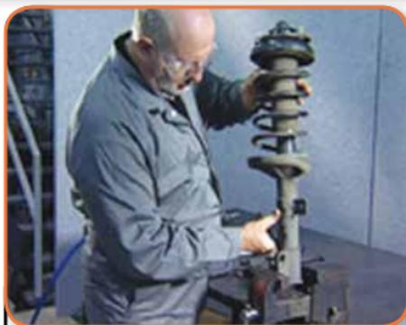
Mount the strut assembly securely in a vice ensuring that you do not damage the casing...
