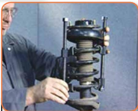
...and attach the spring compressors to the coil springs and compress the coils.
