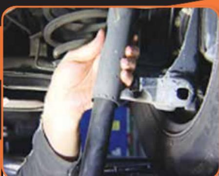
Slide the shock absorber away from the mounting boss and remove it from the vehicle.
