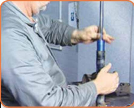
Fit the new strut cartridge into the strut housing...
