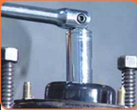
Position the upper cradle and top mount on the shaft and tighten the securing nut.
