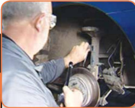
If the shock absorber is part of the whole strut assembly, you will need to remove that first before you can replace the shock absorber.
