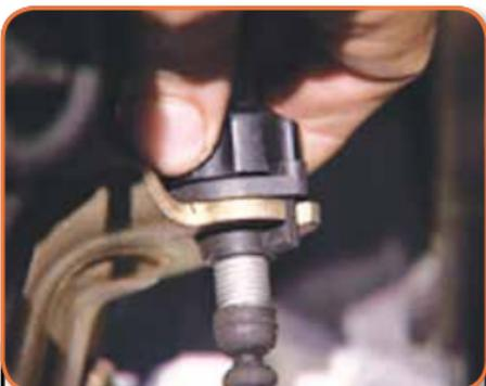
...or by loosening a jam nut on the outer clutch cable and adjusting the cable in relation to its fixture bracket, to the manufacturer's specification...
