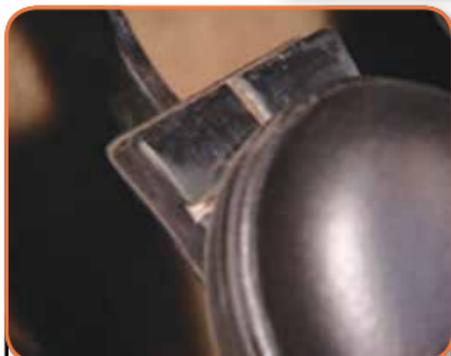
Lightly push down on the clutch pedal, approximately 2.5cm, until it meets resistance.
