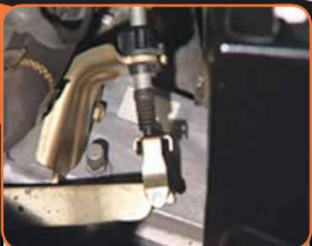
Cable or mechanical systems may require an adjustment to the length of the cable housing. Most hydraulic systems are self adjusting, but those that are not may require an adjustment to be made at the slave cylinder push rod.
