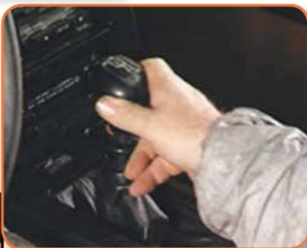
Make a gear selection to ensure the gears do not grate when selected.
