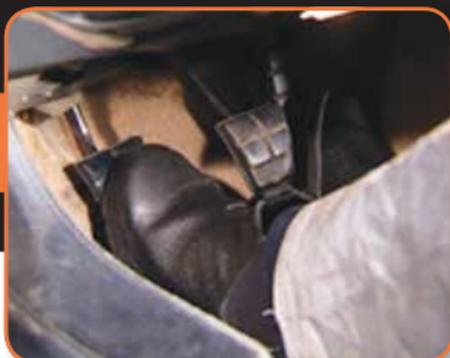
While in gear, slowly release the clutch and see how far the pedal must travel before the clutch starts to take up.
