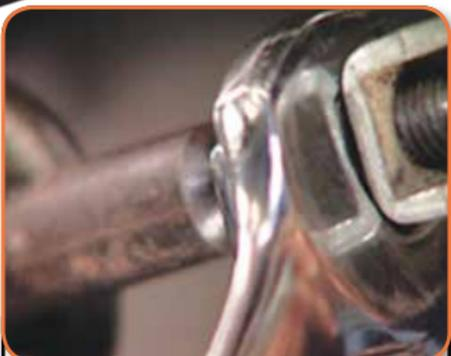
...and then moving an adjusting nut on a rod located on the clutch pivot arm...
