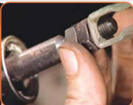
Make the relevant adjustment, which is normally done by loosening a jam nut...
