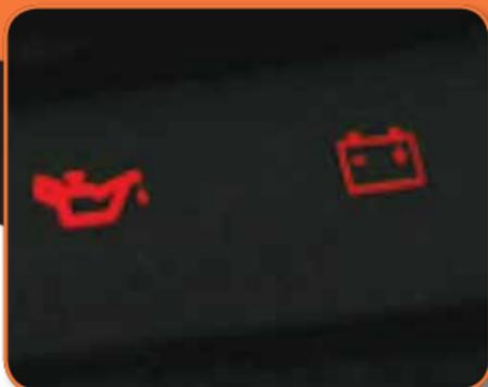
The charge light on the dash should light up, and go out when you start the engine. This indicates that the alternator is charging the battery.
