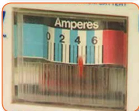
Check the charger amperage output to ensure that the battery is charging correctly. A slow charger usually charges at a rate of less than 5 amperes.
