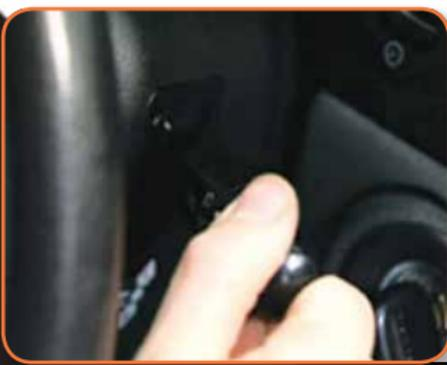
Switch on the vehicle headlights, then start the engine and see if the lights brighten significantly.
