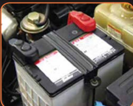
A sealed or low-maintenance battery has no removable cell covers, so you cannot adjust or test the fluid levels.
