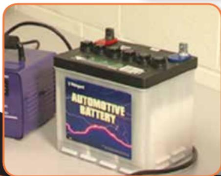
Allow the battery to stand for at least 5 minutes before testing the battery.
