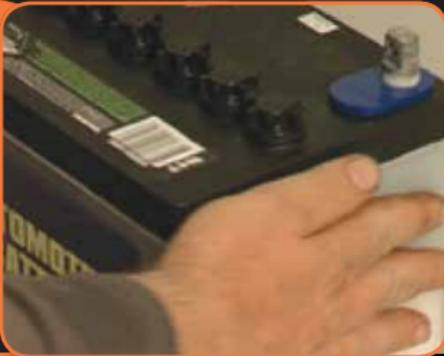
Carry out a visual inspection of the battery to ensure there are no cracks or holes in the casing.
