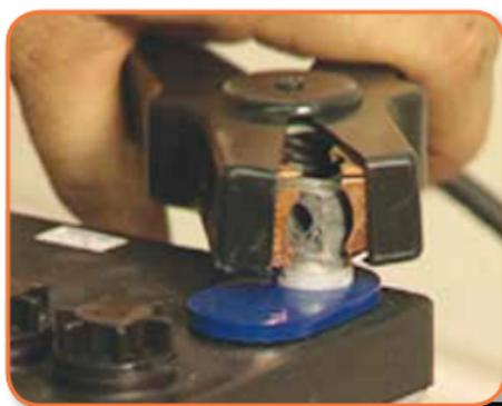
Connect the black lead from the charger to the negative battery terminal.
