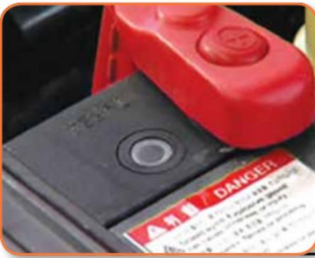
However, some of these do have visual indicators that provide information on the status of the charge and condition of the battery cells.
