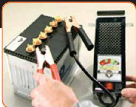
A load tester induces a high rate of discharge in the battery, like the load created by a cranking starter motor. A battery is rated in ampere hours, which means that it can supply a certain number of amperes for a specified length of time under continuous load.
