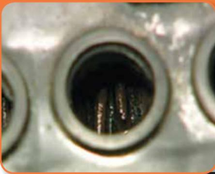
If the level is below the tops of the plates and their separators inside, add distilled water or water with a low mineral content until it just covers them. Be careful not to over fill the cells as they could "boil" over when charging.
