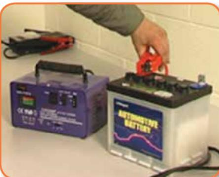
Connect the red lead from the charger to the positive battery terminal.
