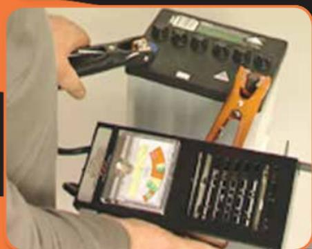
Using a load tester or hydrometer, test the charged state of the battery.
