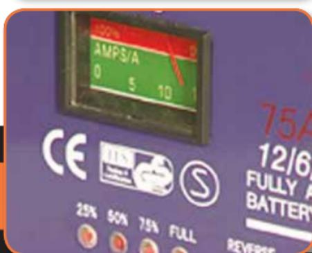
A fast charger charges at a much higher ampere rate, depending on the original battery state of charge and should only be carried out under supervision.
