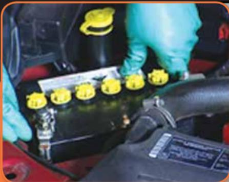
Check that the battery casing and the terminals are in good condition. This can generally be achieved with a visual inspection, however, since the battery may be located in a position where you cannot see all of it, you may have to remove it to complete the inspection, after performing any other on-car tests.
