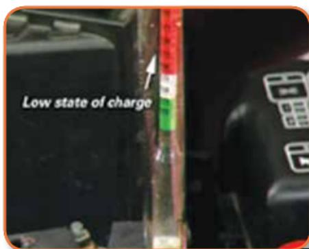
The scale indicates the relative charge state of the battery by measuring how high the float sits in relation to the fluid level. A very low overall reading of 1150 or below indicates a low state of charge.
