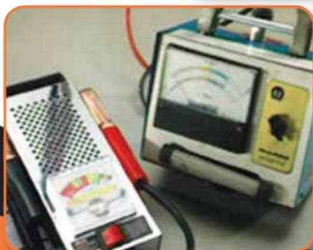
Measure the continuous load capability of the battery with a load tester.
