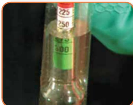
A high overall reading of about 1300 indicates a high state of charge.
