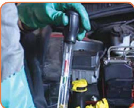
Test the specific gravity of each of the cells by using a hydrometer designed for battery testing. Draw some of the electrolyte into the tester and look at the float inside it.
