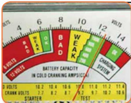
Another measurement used is International Standard Cold Cranking Amps. Check the specifications for the battery you are testing. If it can meet these specifications under a load test then it is in good condition. There are different makes and types of load testers. Always use the equipment that manufacturers recommend for testing procedure.
