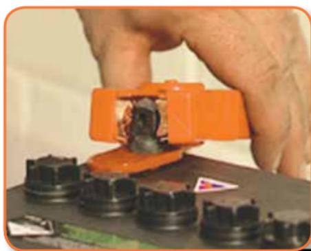
...and the red lead from the positive battery terminal.
