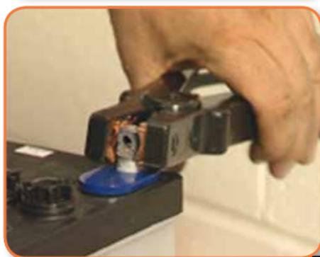
Disconnect the black lead from the negative battery terminal...
