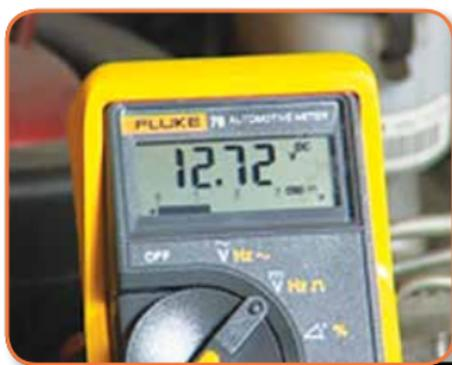
With all vehicle accessories switched off and with the battery at 21 degrees Celsius, the voltage reading should be approximately 12.6 volts if the battery is fully charged. This will be slightly lower at cooler temperatures.
