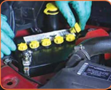
If the battery is not a sealed unit, it will have removable caps or bars on top. Remove them and look inside to check the level of the battery fluid.
